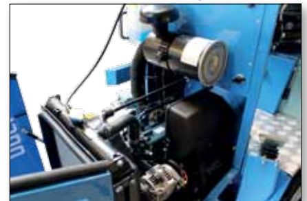
36 BHP Kubota V1505 Engine
