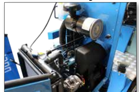
36 BHP Kubota V1505 Engine
